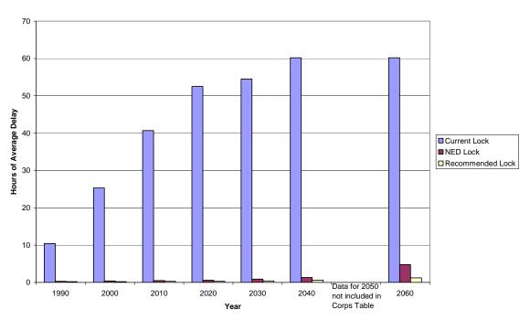
Average Lock Delays at Industrial Canal Lock, Simulation Results from Corps of Engineers 1997 Report
